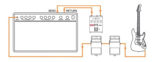
If your amp is equipped with SEND output signal level control then you should set the active reverb LEVEL control to maximum and set in a such way your amp SEND output signal level control to be at the edge of lighting up the DR PEAK indicator (it is recommended to set the amp channels controls at typically used positions and to check all the channels). Then you should adjust RETURN input gain control to receive the same signal level (volume) when the effect loop is active or not.
