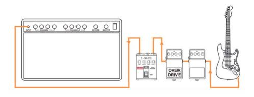
When you use overdrive channel (or channels) of your amp the DR should be connected at the and of the signal path what means, to the amp effect loop.
