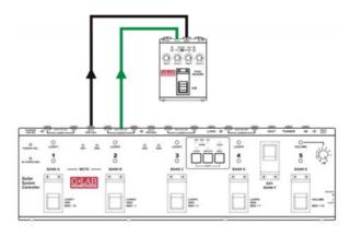
According to the signal (only in case when we don't use the amp's reverb) it is recommended to connect the DR between the GSC and the amp input or to the LOOP4 loop of the GSC. In such a case power supply can be supplied from 9V output of the GSC.
