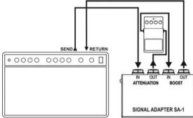
In case of using the looper the way of connecting the adapter to the effects loop with to high signal level is shown below.
