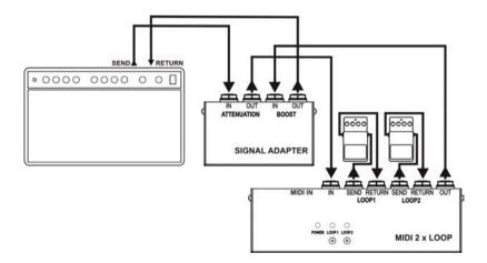
The way of connecting the adapter in order to adjust the signal level (in this case signal attenuation) to one of the effects is shown below.
