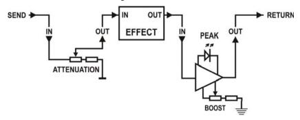
If the signal level is to low adapter enables to reinforce the signal sent to the effect and to attenuate the return signal.
