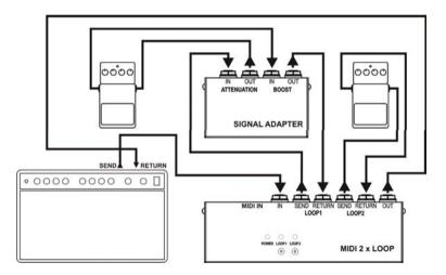
The way of connecting the adapter to the amp effects loop with too low signal level is show below.
