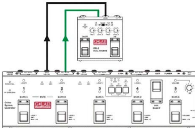
According to the signal (only in case when we don't use the amp's reverb) it is recommended to connect the DR between the GSC and the amp input.
