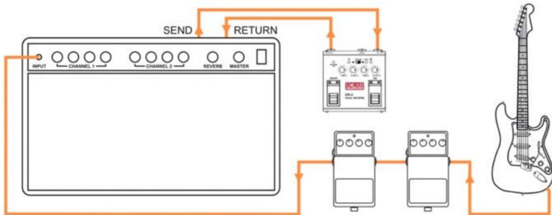
If your amp is equipped with SEND output signal level control then you should set the active reverb LEVEL control to maximum and set in a such way your amp SEND output signal level control to be at the edge of lighting up the DR PEAK indicator (it is recommended to set the amp channels controls at typically used positions and to check all the channels). Then you should adjust RETURN input gain control to receive the same signal level (volume) when the effect loop is active or not.
