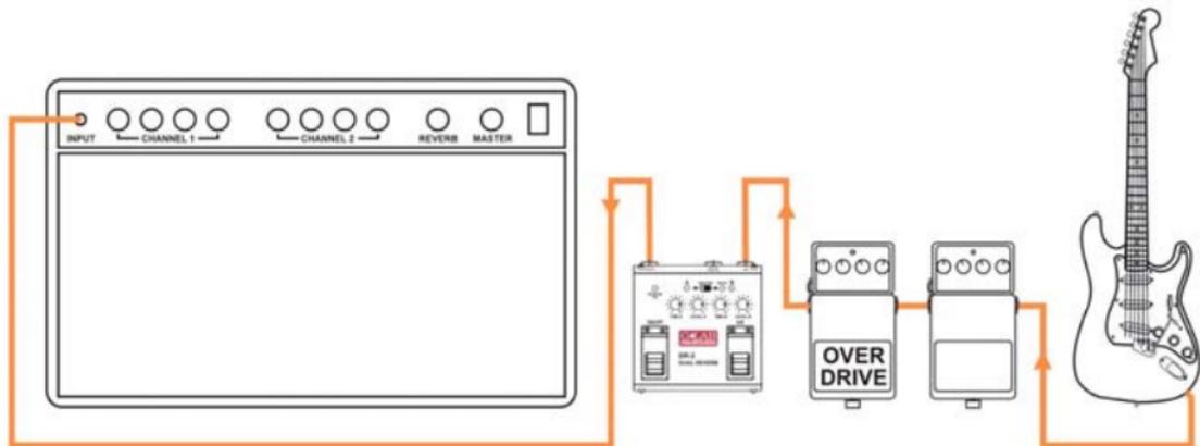
When you use overdrive channel (or channels) of your amp the DR should be connected at the end of the signal path what means, to the amp effect loop.
