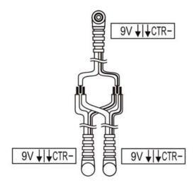
To link the cables you need basic tools and heat shrink tubes (provided with adapter). Strong screwing together the wires and using the heat shrink boot assure reliability and durability of the linking even for three wires.
