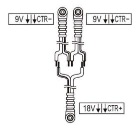
Using separated supply is the basic agent enabling to build the guitar systems without ground loops and supply crosstalk (the influence of variable load of one effect on the second). The best solution is to use separated supply of every effect. The exception from this is possible when the following conditions are met:
