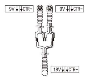
The diagram below shows the cable for supplying the effects requiring 18V DC with polarity CTR + (center positive) (two 9V CTR - inputs, 18V CTR + output).
